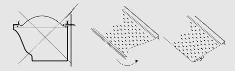
Cut 2 sections as shown below. Make sure you cut the flat end. Follow a line of perforations to cut in a 45° straight line. The template below is on scale.
