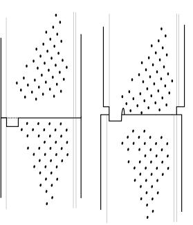
To avoid any overflowing, do not install the Clip N Guard  $^{\rm m}$  on the top of the end cap.
